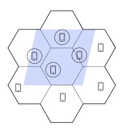
Fig A. Illustrates the process of cell broadcast and Device-Based Geo-Fencing. The blue shaded region represents the target area polygon. This information is transmitted to the Mobile Network Operator (MNO) and then to the Cell Broadcast Center (CBC). The CBC selects the cells that cover the specified target area based on the MNO Policy. Mobile devices determine if they are in the area or not to display the message.
