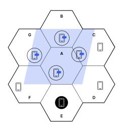
Fig B. Illustrates the process of cell broadcast at a deeper level. As illustrated in Fig A. devices that are in the target area polygon will receive the alert. If devices in cell sites C, F, or D are older or unable to provide their location, they would receive the alert. Phone in cell site E, can share its location but isn't in the targeted area, but if it enters the area within a certain amount of time, it will receive the alert.
